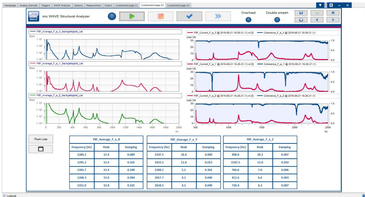
Fig. 4: Diagram on the upper left: Compliance frequency response [Y-axis logarithmic] Diagram on the upper right: transfer function FRF [Y-axis in dB (logarithmic)] tables: Peak-Lists X-, Y- and Z- axis sorted by amplitudes with frequency and attenuation
