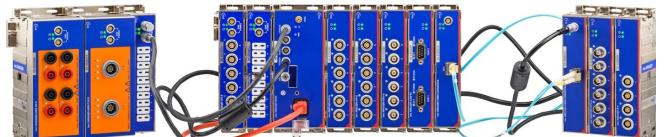
imc ARGUSfit also provides complete integration of the imc CANSASfit module series for slower channels, e.g. for temperature measurement. Such imc CANSASfit modules (CANFT) are likewise internally connected with power and CAN bus and are fully supported and integrated by the software as a uniform system. Finally, imc CANSASfit modules can even be installed in distributed topologies and connected via CAN-cable to the imc CANSAS-Interface of the base unit.
