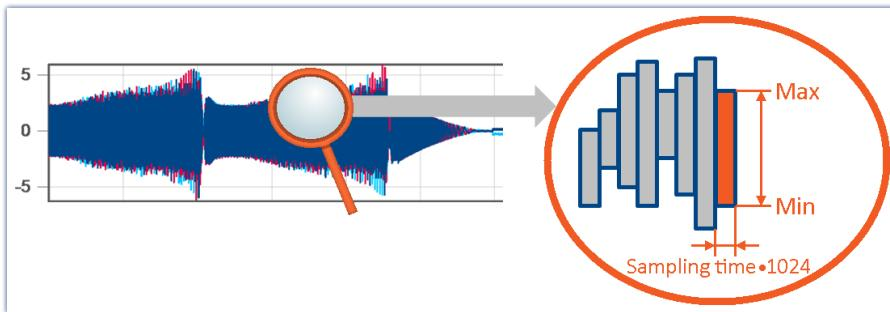
Envelope type monitor channels are available on the Setup page: "Analog Inputs" under the channel type: "Monitor Channels". The "preprocessing" must be set to "Envelope".
