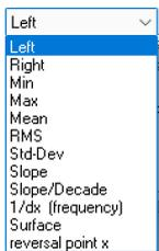
By default, the columns display the content shown in the image 1. Additionally, the standard deviation and the RMS-value of the readings between the measurement cursors can be displayed.
