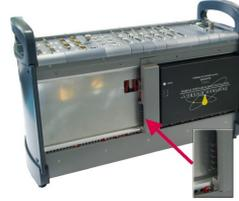
*imc CRONOScompact with two Li-ion battery packs*
