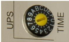
Both handles (CRFX-HANDLE-LI-IO-L and the CRFX-HANDLE-UPS-L) are equipped with a switch to set the buffer duration (table).
