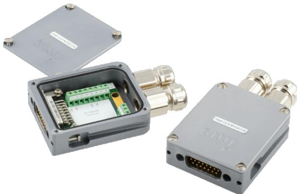
The two PFLITSCH M12 x 1.5 cable connections seal cables with a diameter from 6.5 mm up to 9.5 mm.
