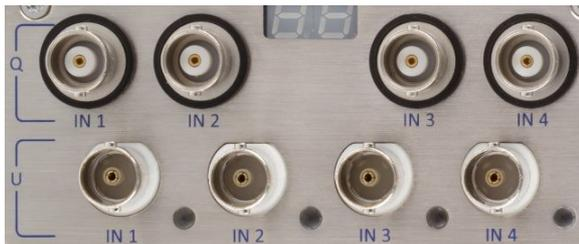
The connection is made via eight BNC sockets, four of which are for voltage measurement or optionally for ICP (**U**) and four for charge measurement (**Q**). The connections are labeled accordingly: U or Q
