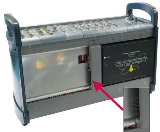
*imc CRONOScompact with two Li Ion battery packs*
