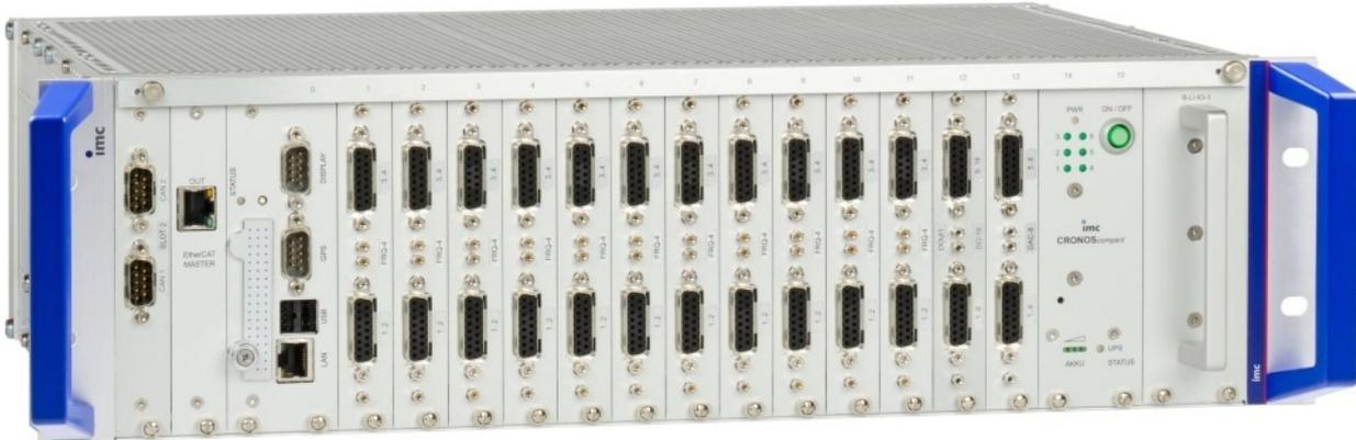
There are 16 free slots in a CRONOS*compact* AC- and DC-RACK. Your system can be freely configured with analog, digital and fieldbus modules. Exception #1: totally 16 analog or 16 digital modules, e.g. 16 analog and two digital modules. Exception #2: the [SYNTH-8](#)<sup>317</sup> module, this module will be detected as a fieldbus module.
