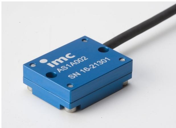
The capacitive accelerometers are based on micro-electromechanical systems (MEMS technology) and allow static measurement of acceleration forces from 0 Hz upward. The scope of application possibilities includes the fields of vehicle dynamics, endurance strength testing, vehicle inspections, brake testing, driving comfort measurement, structure monitoring, or in general wherever reliable measurement of acceleration is needed.
