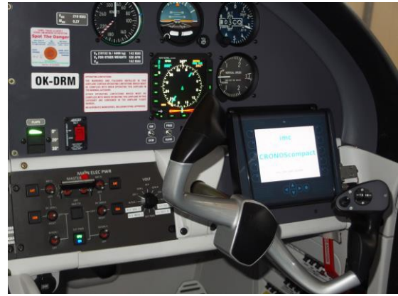
imc 显示器直接固定在驾驶舱内, © Photo: Evektor
